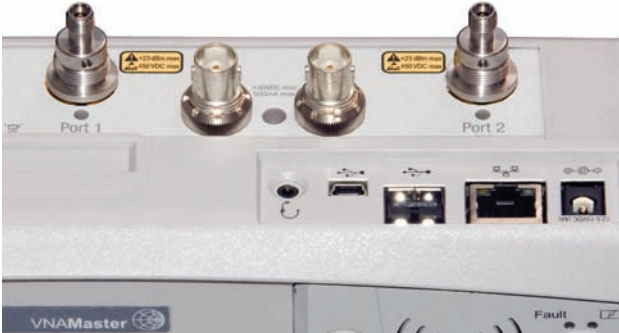
Optional K(f) test port connectors are available for precision measurements to 20 GHz.
