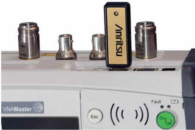
For secure environments, VNA Master will only use external USB memory as an external drive for storage when configured with Option 0007. Internal memory is disabled for data storage.
